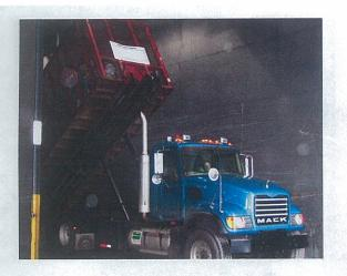
(Above) One of the county's recycling trucks dumps in a bin on the tipping floor, all incoming material is stored in bins until it is fed onto a conveyor belt and sent up to the sorting room where the material is sorted and dropped into bins below. Once the material is sorted it is loaded onto another belt which feeds the Nexgen two-ram baler.
