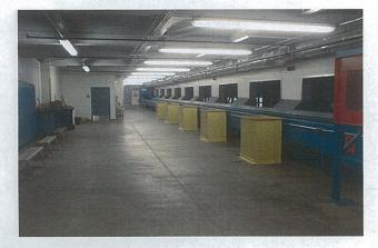
(Below) The cardboard processing area of the building. Here all of the cardboard is sorted and the clean material is baled in a single ram baler making around a 2000 lb. bale. The county processes and ships approximately 66 tons of cardboard a week.
